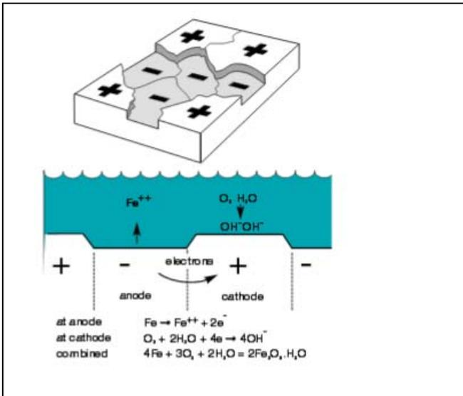
[1] Fig. 1: Mechanism of corrosion
