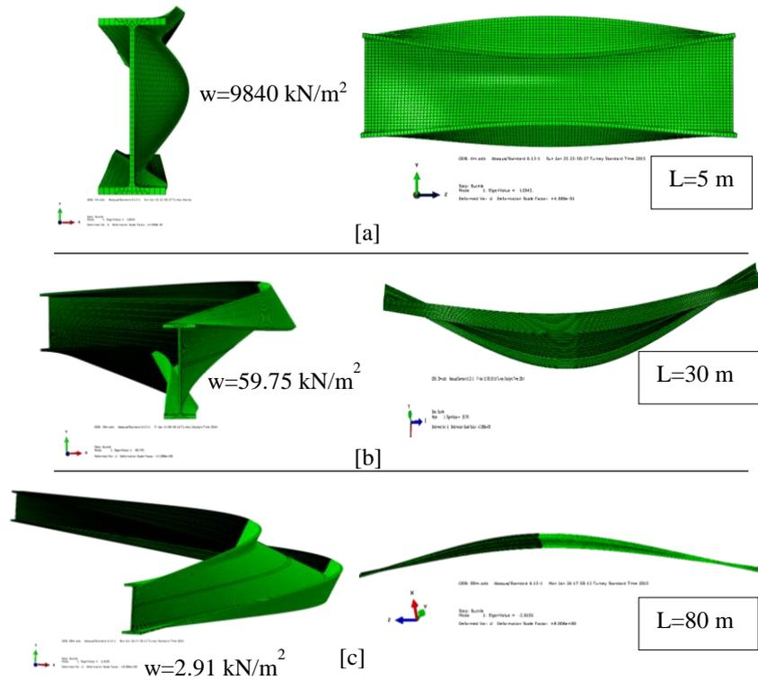
Fig. 4 Buckling analysis results of W44x335.
