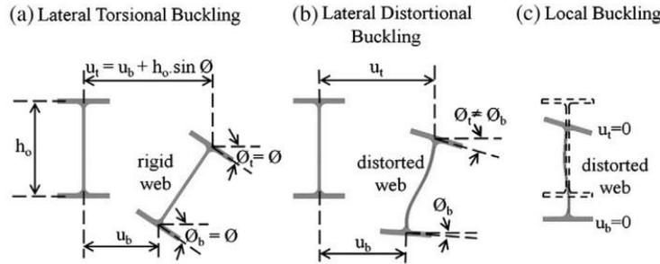
Fig.1. Typical buckling modes of I beam [13]
