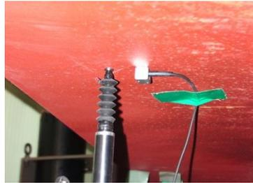
(b) Displacement-transducer and accelerometer
