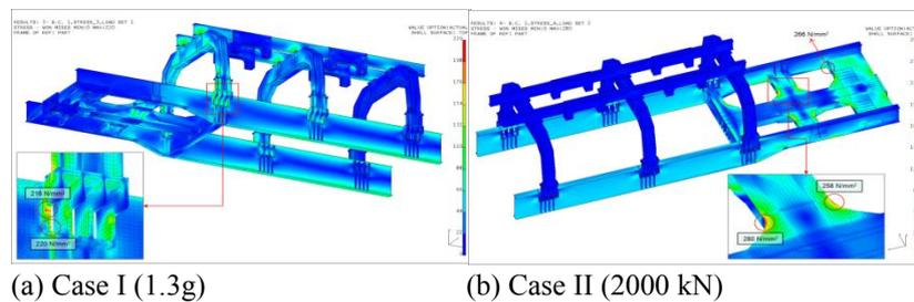
Fig. 4. Analytical results of the crane vehicle
