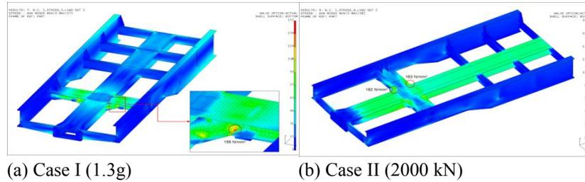
Fig. 3. Analytical results of the carrying vehicle
