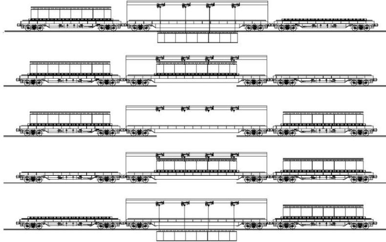
Fig. 2. Procedure for replacing the existing superstructure of an OSPG bridge
