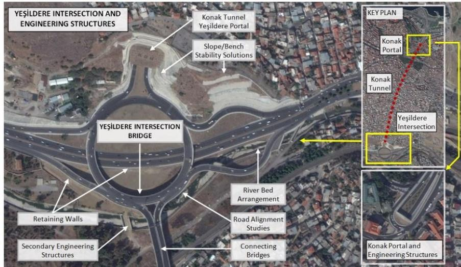
Figure-1: Overall project site showing engineering structures
