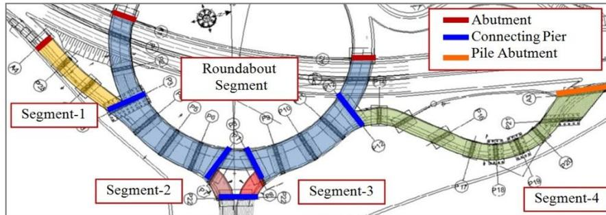
Figure-2: Yesildere Intersection Bridge General Layout
