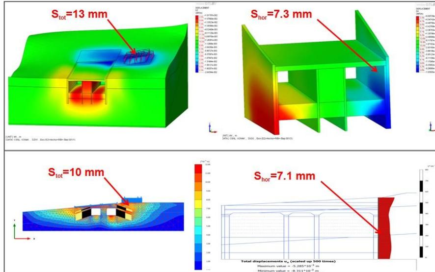
Figure-4: Konak Portal Top-Down Culvert Analyses Results
