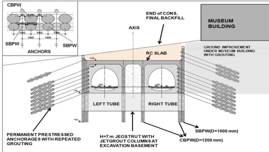
Figure-3: Konak Portal Top-Down Culvert Typical Section
