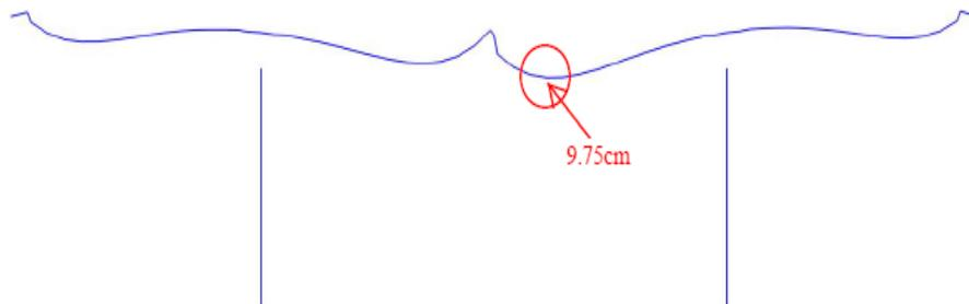
Construction stage no.20, displacement curve (36000days-100years)
