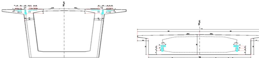
The post-tensioning tendons so determined were defined in the model placing them in suitable positions (Figure 6) and as a result of the analysis, concrete stresses and deformations in the deck sections were checked. Transverse post-tensioning tendons had to be used since the width of the bridge is 17m. These tendons also were defined in Midas Civil Program.
