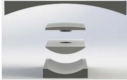
*Figure 7. Representation (exploded view) of designed bearing – with central two-part calotte having cylindrically shaped upper and lower sliding surfaces.*
