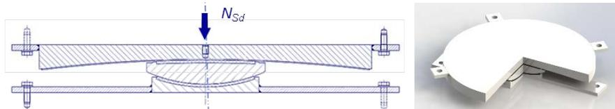
Figure 3. Cross-section and cut-out view of a typical pendulum isolator bearing.
