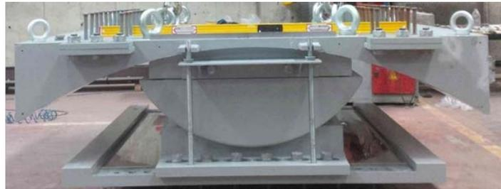
*Figure 9. A “cylindrical” pendulum bearing, as fabricated.*
