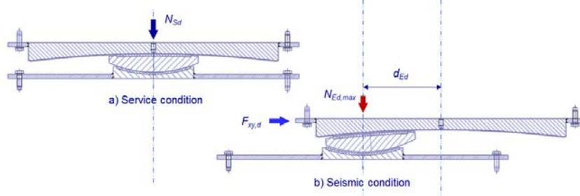
Figure 5. Cross-sections of a typical pendulum isolator bearing showing how it facilitates horizontal ground movements (in any direction) during an earthquake.
