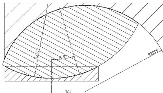
Figure 6. Cross-section if designed as a standard pendulum bearing – with central calotte having spherically shaped upper and lower sliding surfaces.
