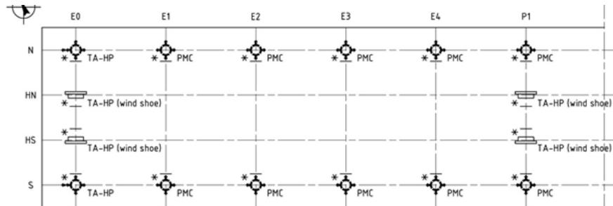
Figure 2. Bearing scheme of a side span of the bridge (elevation and plan). PMC indicates a pendulum bearing, while TA-HP indicates a pot bearing.
