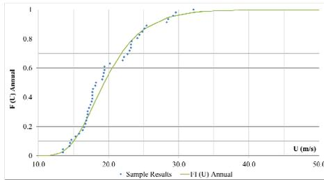
Figure 2 - Cumulative Distributions for the Sample of Annual Maximum and for the adjusted Gumbel Distribution
