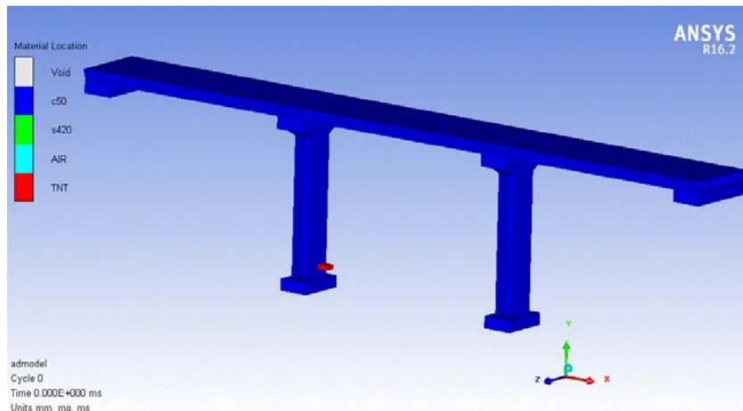
**Fig. 3.** 3D finite element model of the highway bridge
