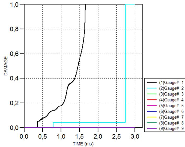
**Fig. 10.** The time histories of the damage on the gauge point
