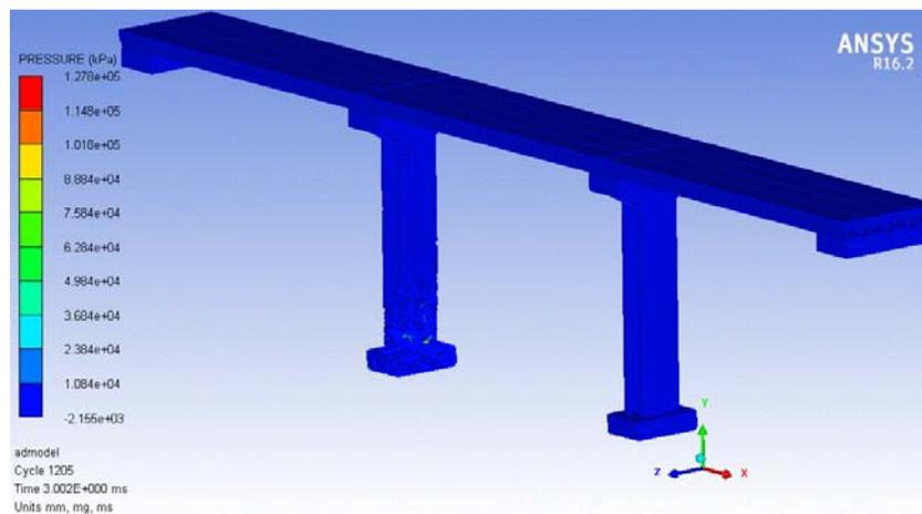
**Fig. 8.** Pressure values of the highway bridge obtained from blasting analyses
