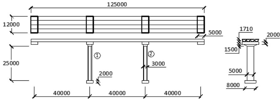
**Fig. 4.** Dimensions of the highway bridge, (units are mm)
