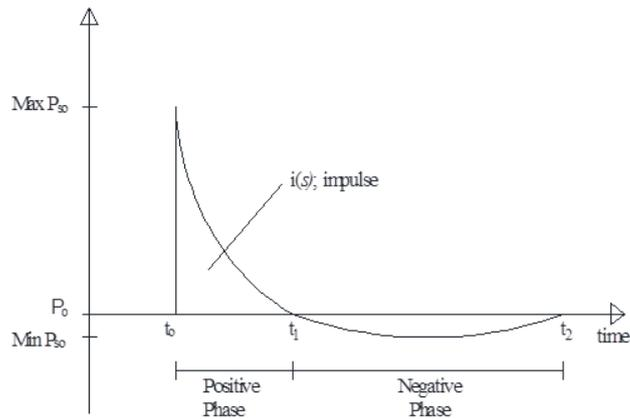
**Fig. 1.** Pressure- Time graph of the explosion [12]
