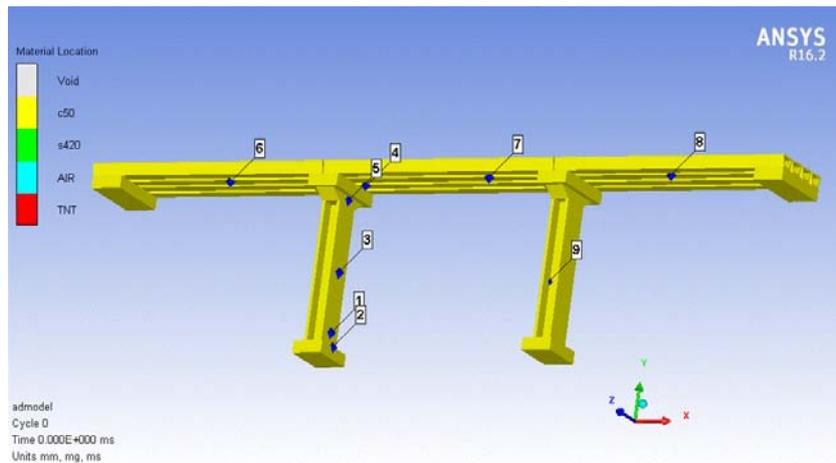
**Fig. 6.** Plotted gauge points on the 3D finite model
