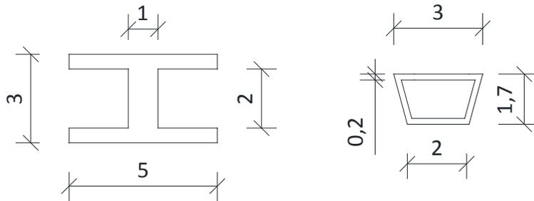
**Fig. 5.** Cross sections and dimensions of the column and beam, (units are m)
