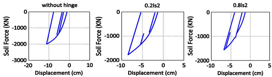
Fig. 6 The backfill soil response under the near-fault earthquake.
