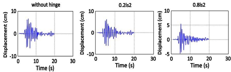
Fig. 4 The deck displacement along longitudinal under the far-field earthquake.
