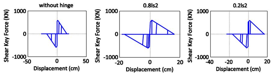
Fig. 7 The shear key response under the near-fault earthquake.
