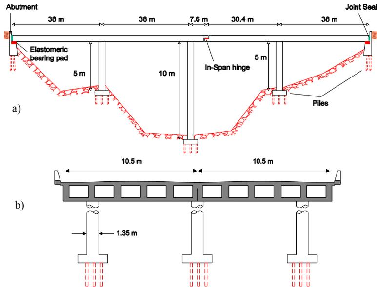
**Fig. 1** A general view of the multi-frame concrete box-girder bridge in: a) longitudinal direction, and b) cross-section.
