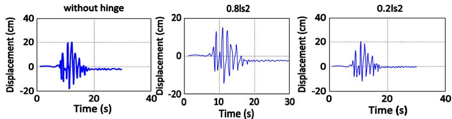
**Fig. 3** The deck displacement along longitudinal under the near-fault earthquake.
