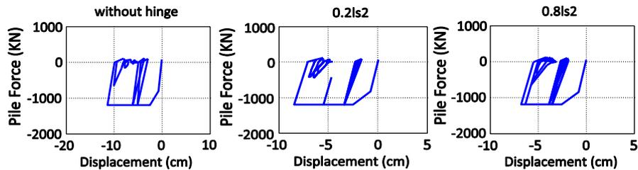
Fig. 8 The abutment pile response under the near-fault earthquake.
