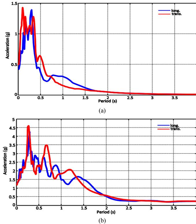
**Fig. 2** Response spectrum of the a) near-fault and b) far-field ground motions selected for this study in transverse and longitudinal horizontal directions.
