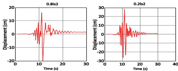
Fig. 5 The deck displacement along transverse under the near-fault earthquake recorded at the in-span hinge location.
