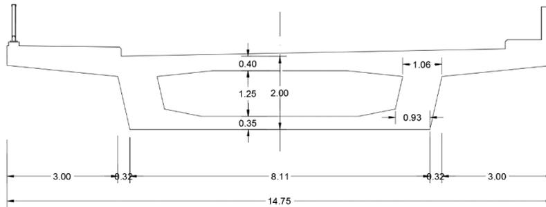
Fig. 2. Cross-section of superstructure at mid-span
