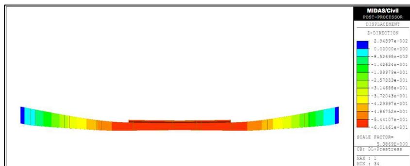
**Fig. 9.** Vertical deflection of bridge under posttensioning and dead loads.
