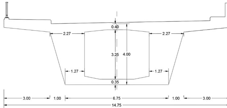
Fig. 1. Cross-section of superstructure at abutments
