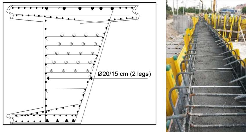
**Fig. 5.** Shear reinforcement at anchorage zone and interface between web and slab
