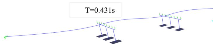
Figure 4 First mode shape of the bridge with 30m span length for soil type 3.
