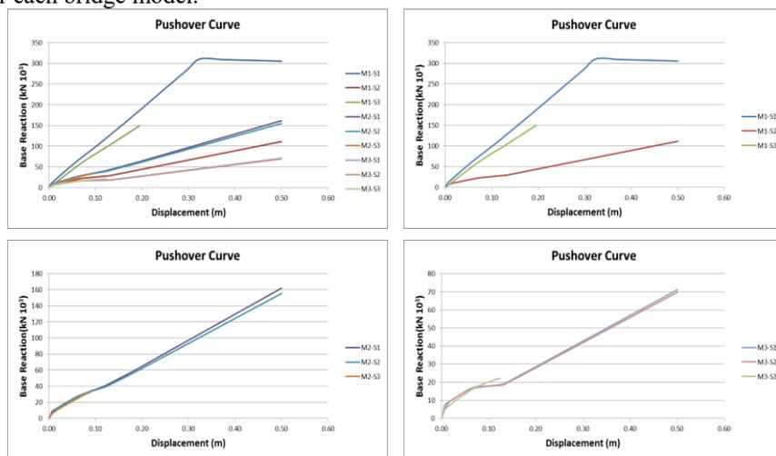
Figure 5 Pushover Curves for lateral directions of the bridges
