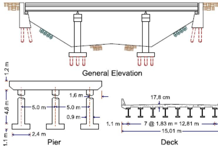
**Figure 1 View of multi span continuous bridges [18].**
