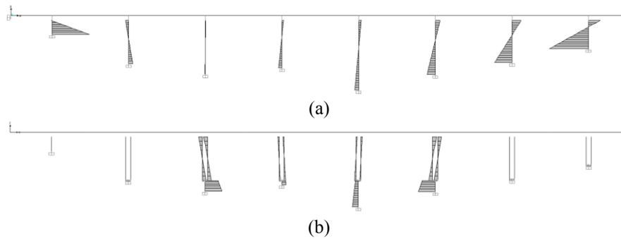
Figure 12. Eyiste Viaduct pier moment diagrams due to uniform temperature change (a. initial design; b. modified model)
