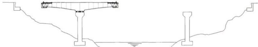
Figure 2. BCM during cantilever construction [1]
