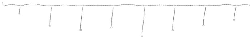
Figure 5. Eyiste Viaduct deformed shape under longitudinal seismic force.
