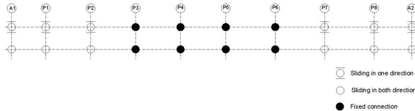
Figure 8. Eyiste Viaduct modified bearing conditions
