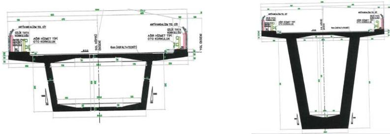
Figure 4. Eyiste Viaduct typical deck cross-sections
