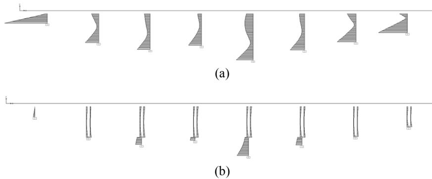
Figure 10. Eyiste Viaduct longitudinal seismic force moment distribution (a initial design; b, modified model)
