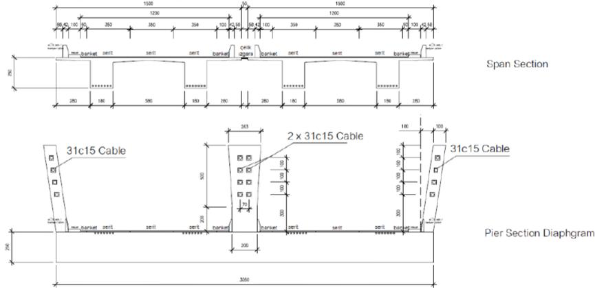
Figure 5. Typical cross-sections of Çallı Bridge
