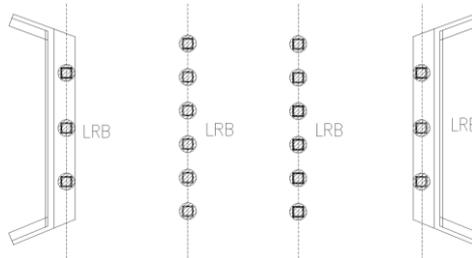
Figure 6. Bearing layout of Çallı Bridge
