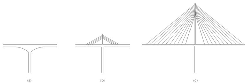
Figure 2. Typical view of (a) girder, (b) extradosed and (c) stay-cable bridges
