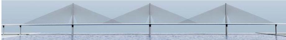
Figure 10: Example of a continuous cable stayed bridge [4]
