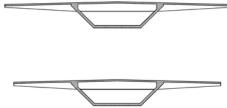
Figure 8 Cross section with different widths and transversal cross beams.
