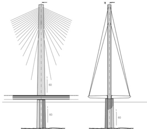
Figure 4: Central pylon with lateral suspended deck.
