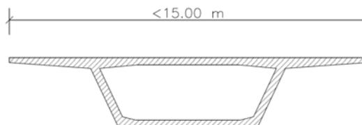
Figure 6: Narrow cross sections, without ribs or struts
